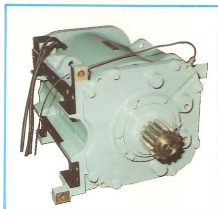
(Left) A nose-suspended dc traction motor supplied for light rail duties. (Above) A three-phase induction motor which was designed to be mechanically interchangeable.
