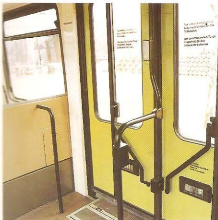
Passenger access can be from either high level platforms or from street level.
