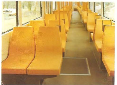
An alternative arrangement with 2 x 1 seating gives more space for standing passengers.
