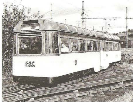
A vehicle evaluating three-phase, off-vehicle control is seen on the Company's test track in 1983. The layout of the test track is shown (left).
