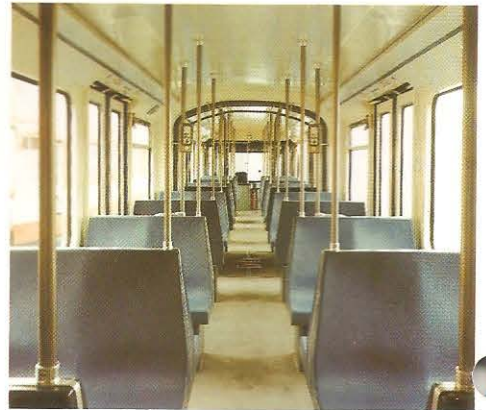
A typical interior layout with 2 x 2 seating (which gives probably the highest proportion of seated passengers).
